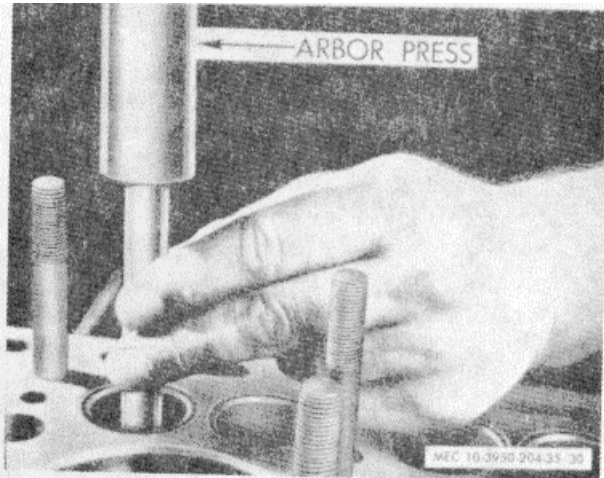
Figure 30. Removing valve guides.
